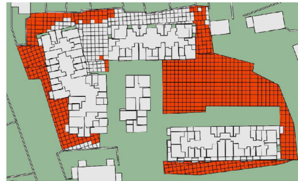
Proposed Development Amenity Areas – March 21 st Cells coloured red if they receive ≥2 hours of sunlight 78% of Amenity garden area receives ≥2 hours of sunlight, therefore the BRE Guideline is Achieved
